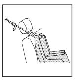
If the position you are using has an adjustable head restraint and you are using a single tether, route the tether under the head restraint and in between the head restraint posts. See Head Restraints on page 13.
